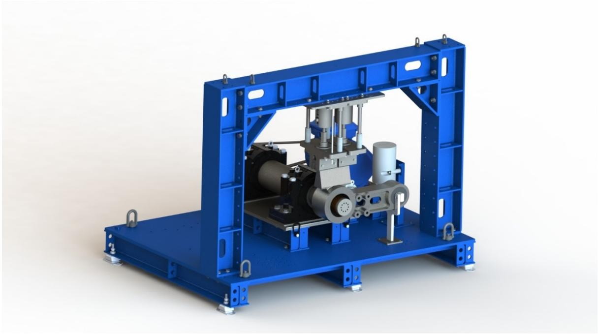
*Bearing test rig for characterising vibration under load and at speed.*
