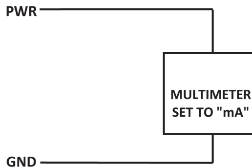
Figure 4. Measurement of output current during installation (use multimeter cable #66562)
